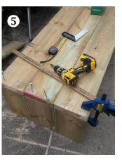
ADD SIDES Fix the first short side to the long sides with torte screws. Repeat to build the other side.
